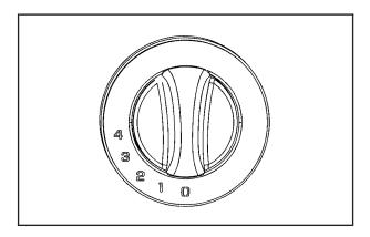
The panoramic sunroof control is located on the headliner. From the closed position, turn the control clockwise to vent the sunroof or open it to three different positions.
